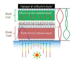
**Fig.** Schematic device structure of Perovskite (Front cell) with bi-functional encapsulation (back cell) tandem solar cell in series connection to solve the degradation issues resulting from moisture and oxygen.
