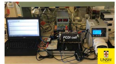
Composite current collector for FCDI and a bench-scale FCDI system
