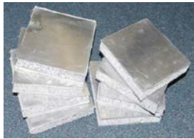
New composite sandwich panels Skin-fibre metal laminates Core-aluminium foam
