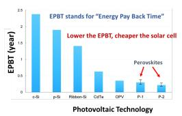
Energy payback time for seven PV modules. P-1 and P-2 represents Perovskite module with different material systems. Organic and perovskite PV technology are the cheapest means of solar power. Source: Jian et al. Energy Environ. Sci., 2015, 8, 1953-1968
